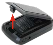
Step 2 Open the cover of battery
