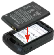
Step 4 Fit new battery into GPS-4013
